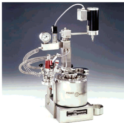
Figure 8. Premex miniautoclave. Reproduced with permission from premex reactor gmbh. 154
